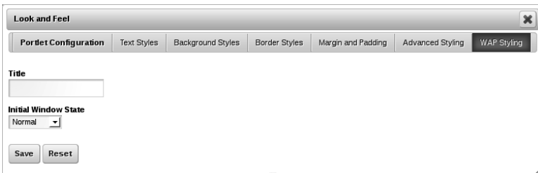
Figure 7.7: The WAP Styling tab lets you enter a custom portlet title to be displayed to devices making page requests via WAP; it also allows you to specify an initial window state.
