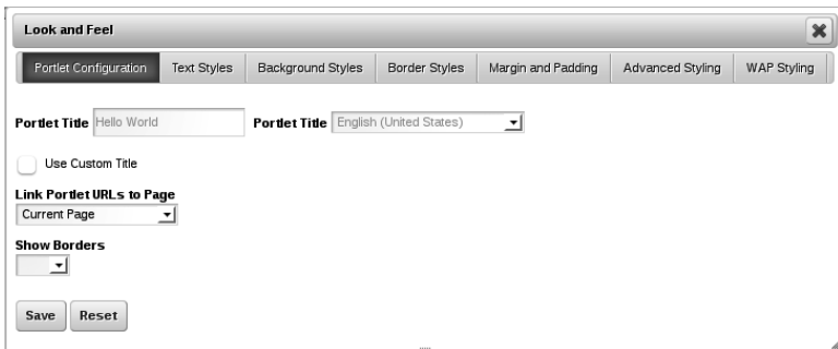
Figure 7.1: The Portlet Configuration tab of the Look and Feel Box allows you to define a custom portlet title, link portlet URLs to a specific page, and select whether or not portlet borders should be displayed.
