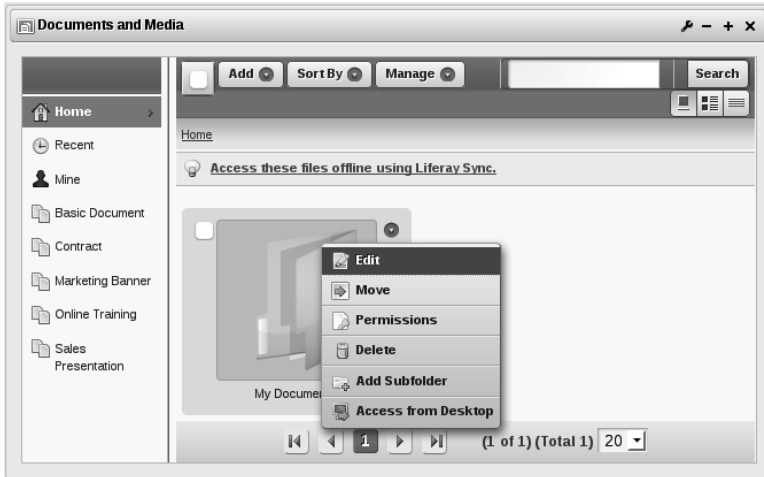
Figure 10.9: Workflow for Documents and Media must be enabled at the folder level. Edit a folder to select a workflow.
