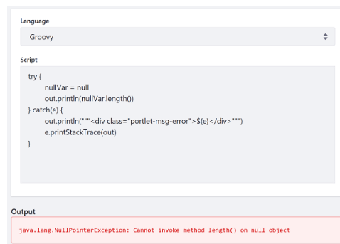
Figure 26.2: Here's an example of a Groovy script that catches exceptions and prints exception information to the script console.
