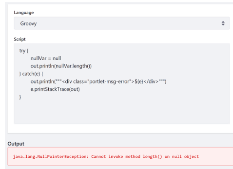
Figure 77.4: Here's an example of a Groovy script that catches exceptions and prints exception information to the script console.
