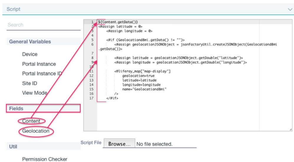
Figure 12.10: Add the Content and Geolocation snippets to quickly create your web content template.
