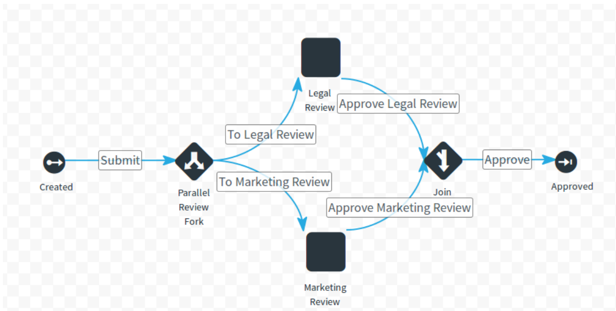
Figure 26.9: Forks and Joins are used to enable parallel processing in the workflow.
